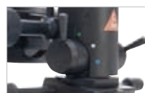
3 different apertures, integrated red-free and cobalt blue filters.
